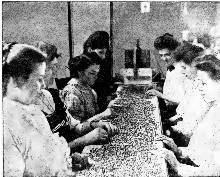
The Final Process —Inspecting the graded shelled seed corn before it is sacked. Any ill shaped or off colored grains that have escaped the grading process are removed here.
